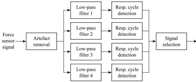
Fig. 2. A flowchart description of the method.
